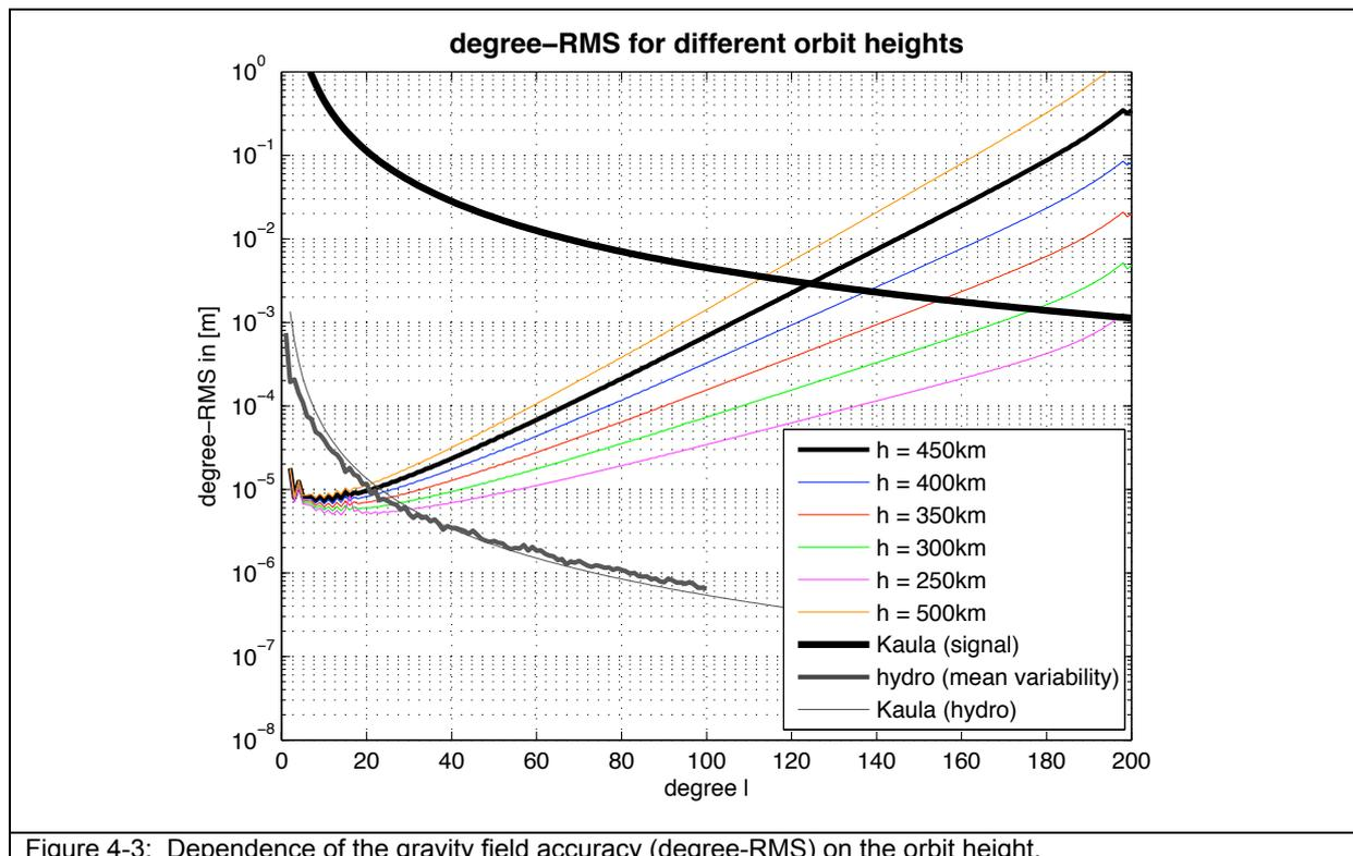
Figure 4-3: Dependence of the gravity field accuracy (degree-RMS) on the orbit height.
