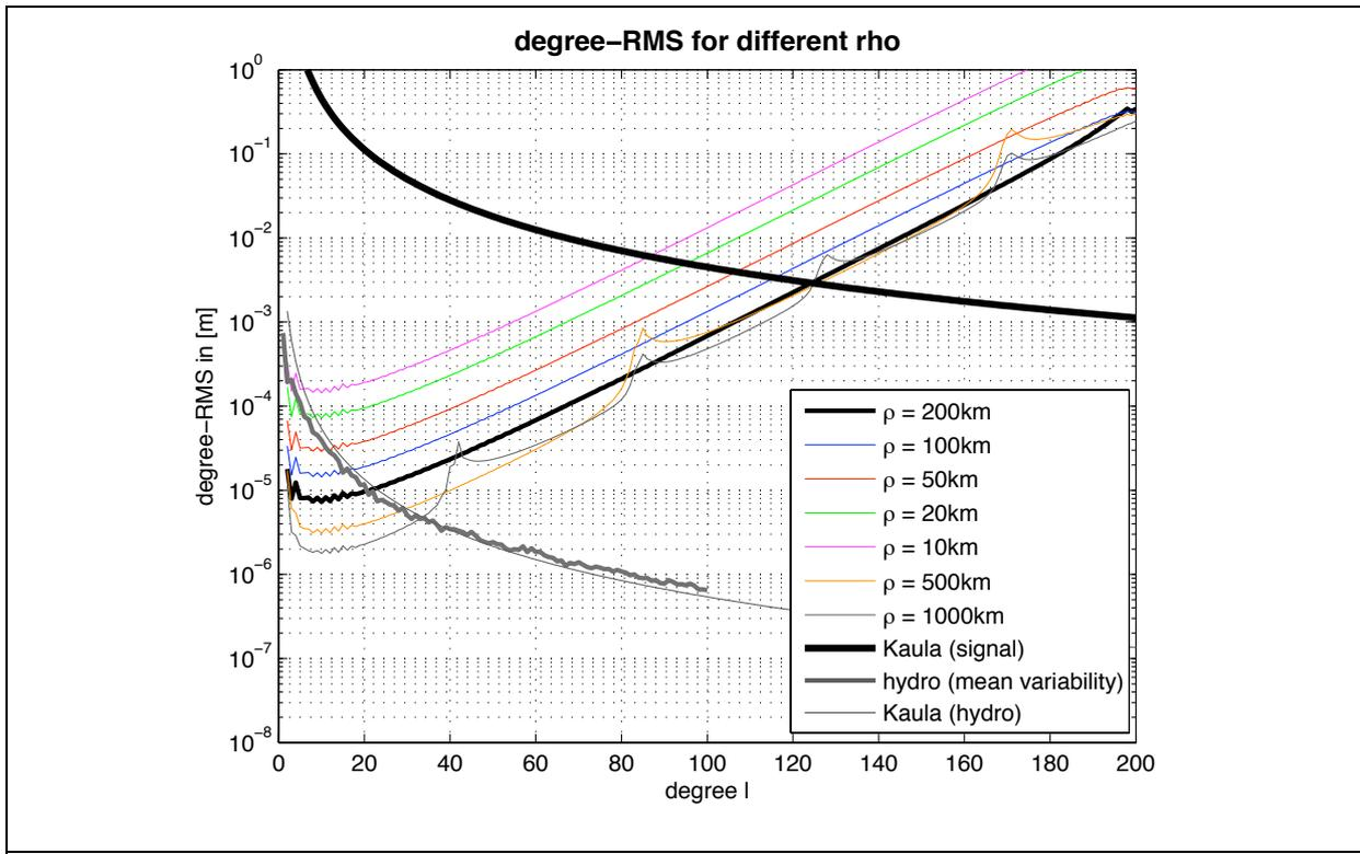
Figure 4-4: Dependence of the gravity field accuracy on the inter-satellite separation distance,  $\rho$ .
