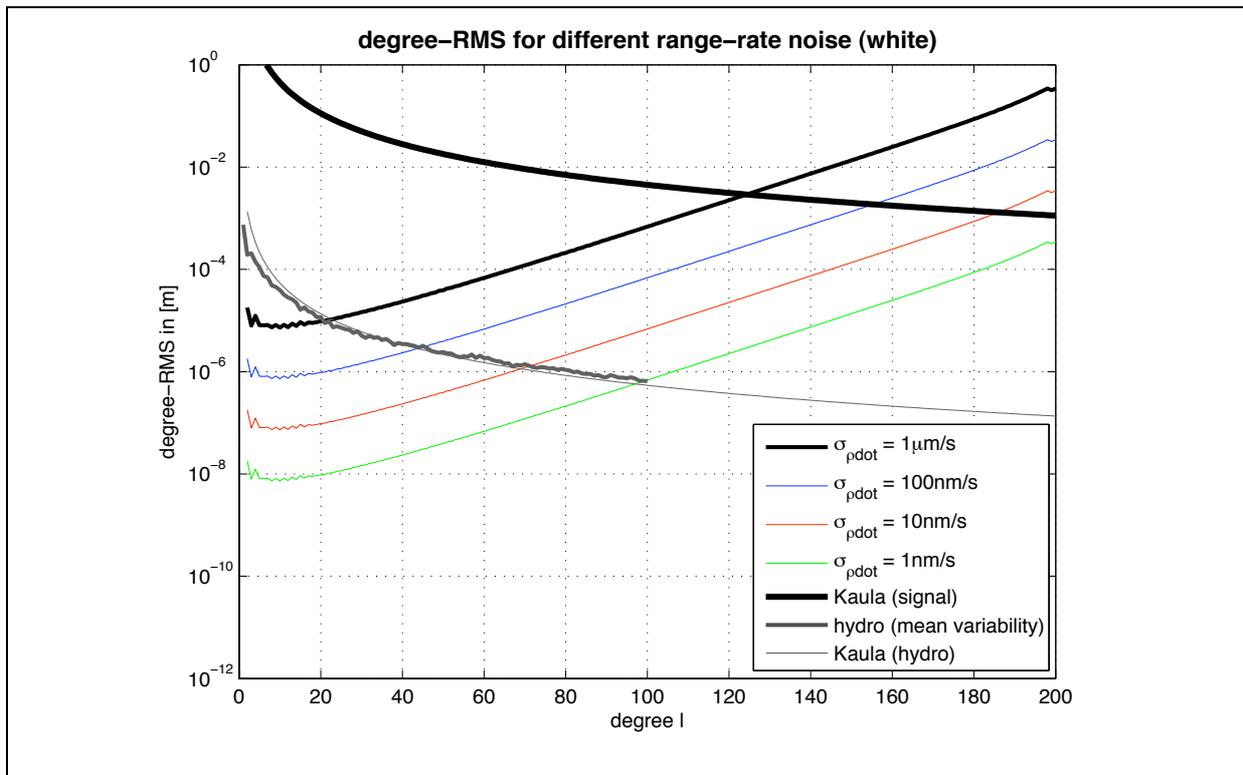
Figure 4-1: Dependence of the spatial resolution on the accuracy of the sensor system (here: k-band/laser ranging).
