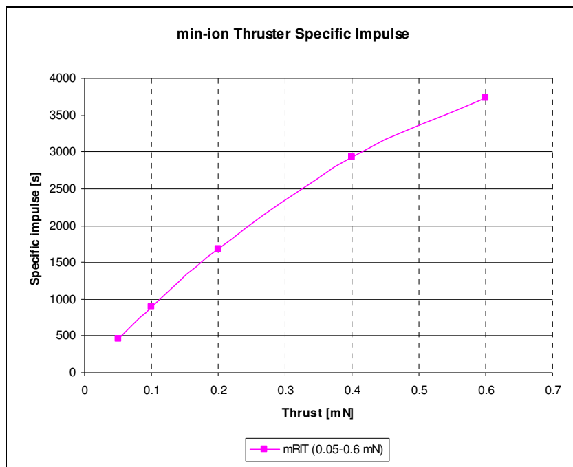
Figure 4-4: Mini-ion thruster specific impulse
